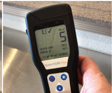
After Simix: ATP reading after cleaning with Simix is 5. The CDC accepts ATP readings as an objective measurement of the cleanliness of surfaces. Anything less than 10 is considered sterile in operating rooms, ICU, and sterile services.
