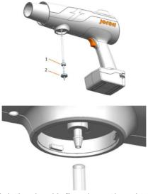
3. Screw on the bottle again, and the filter replacement is completed.
