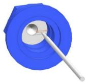
4. According to the assembly diagram, screw on the nozzle core clockwise with a flat-blade screwdriver.
