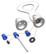
Carefully scrape off the debris and stains on the nozzle with a needle, especially those foreign matters in two grooves on the inner side of nozzle.
